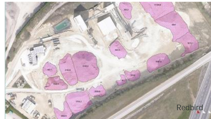
Stockpile maps created from aerial photo surveys provide faster & more accurate volumetric calculations for mining and quarry operations.
